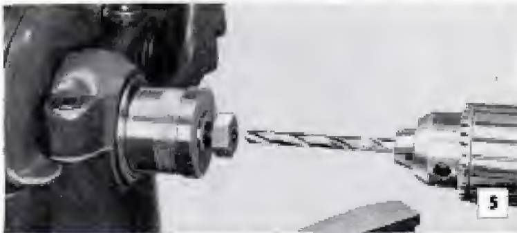
Drilling the pivot bolt axially also can be done in the lathe or drill press. Hole is for insertion of \frac{1}{4} -in. attachment bolt
